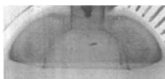
Figure 4: Secondary flow in the upper part of an eccentric spherical gap
